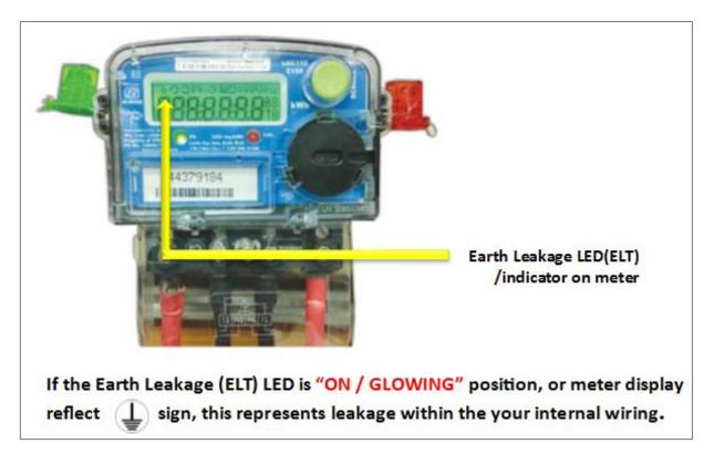
To avoid the hassle of checking the meter for earth leakage every now and then, ELCB should be installed. As ELCB automatically trips and disconnects the electricity supply to the premise / equipment at the detection of earth leakage, thus preventing any untoward incidents. Another, useful benefit of installing an ELCB device is that it also detects faulty and intermixed internal wiring.
