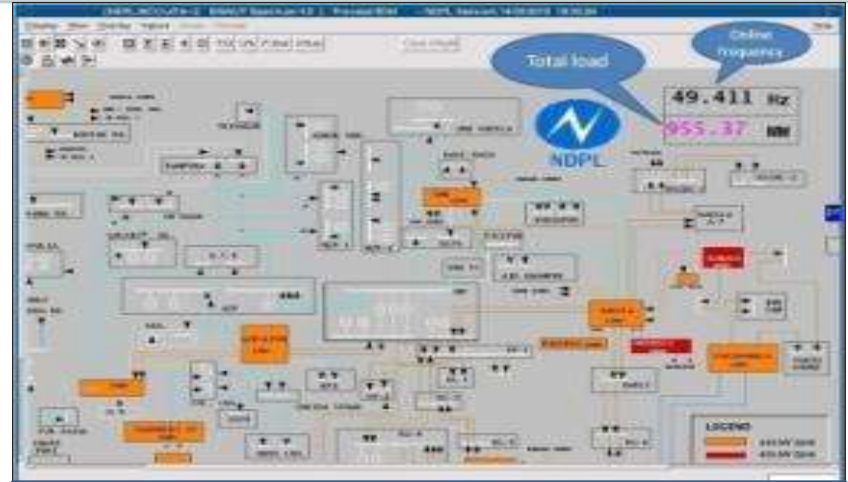
Monitoring of total load through SCADA
